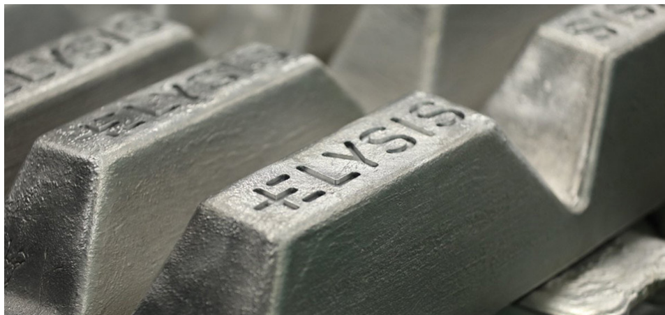
Aluminium ingots made from an electrolysis process almost free from GHG emission
